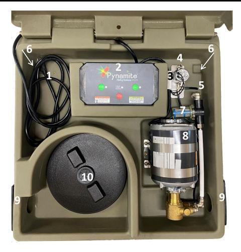
1. POWER CORD – plug into a standard 120v GFCI protected outlet.
