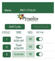
**Cycles 1 & 2 - Dawn & Dusk:** are a convenient way of not having to reset mist cycles with Daylight Saving Time. Dawn & Dusk cycles cannot be deleted only turned ON or OFF.
