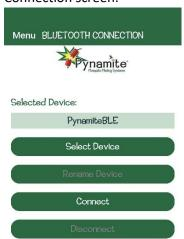
The Selected Device box will show the name of the device that the app is currently connected to. If no device is connected, the field will be blank.
